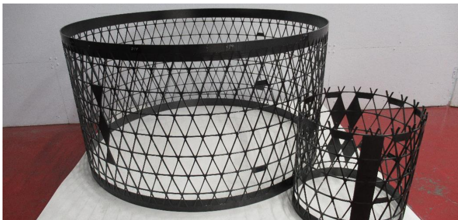
Figure 6: Large cylinder as manufactured, shown here with the small cylinder.
