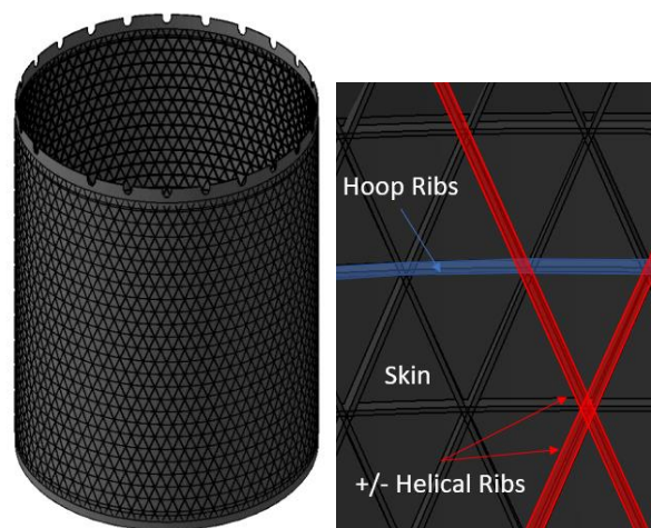
Figure 2: Image of the grid-stiffened interstage component along with an outline of the structure's main constituents.
