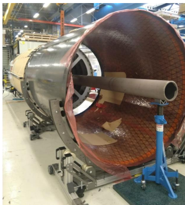
Figure 9: Image of the demoulding process with the extended shaft and part removed from the mandrel.
