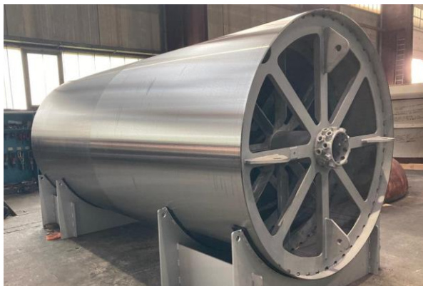
Figure 5: Metallic mandrel for part layup.
