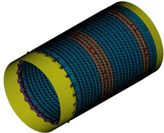
Figure 7: Overall model of the first stage interstage model, including adjacent structures
