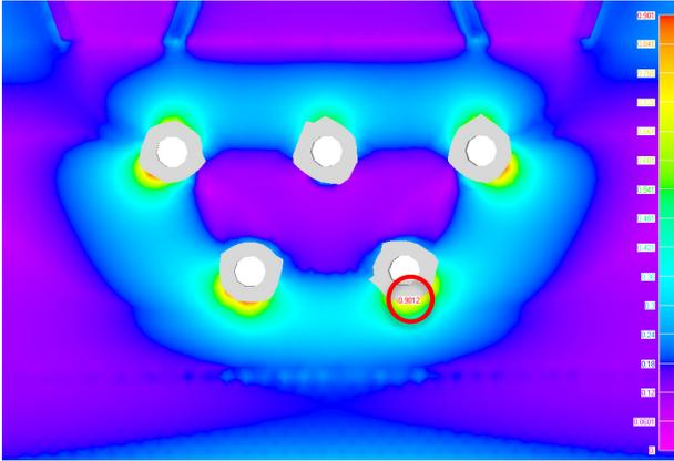
Figure 15: Maximum failure index in the end laminate detailed model (excluding unrealistic results) for the long interstage
