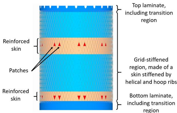
Figure 4: Long interstage design, cut view from inside
