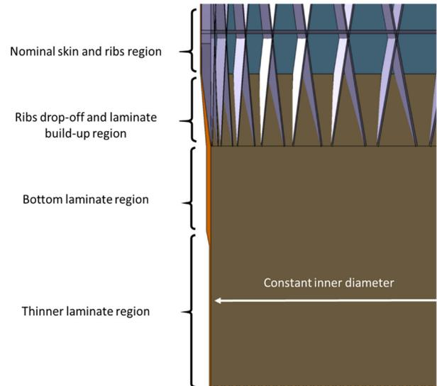
Figure 5: Architecture of the lower laminate region
