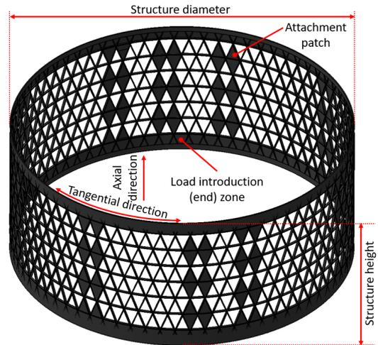
Figure 3: Lattice structures terminology
