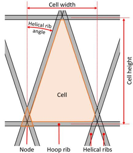
Figure 2: Lattice structures terminology
