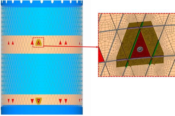
Figure 13: Detailed model for the tank patch analysis of the long interstage model
