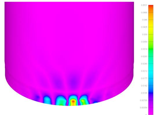
Figure 14: Buckling mode -showing total displacement- for the long interstage global model
