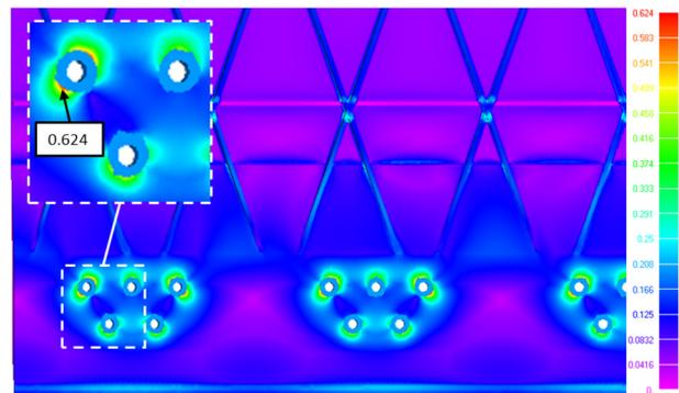
Figure 18: Maximum failure index in the solid tank patch detailed model for the short interstage
