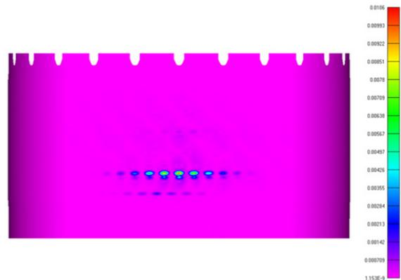
Figure 17: Buckling mode -showing total displacement- for the short interstage global model
