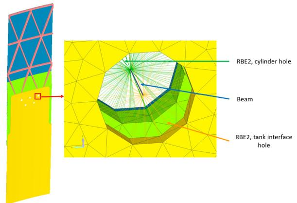
Figure 12: RBE2 and beam elements connecting the tank interface to the bottom end laminate detailed model
