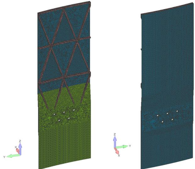
Figure 11: Detailed model of the end laminate for the long interstage design. Blue: skin plies, orange: ribs, green: laminate plies
