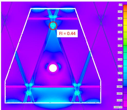
Figure 16: Maximum failure index in the solid tank patch detailed model for the long interstage
