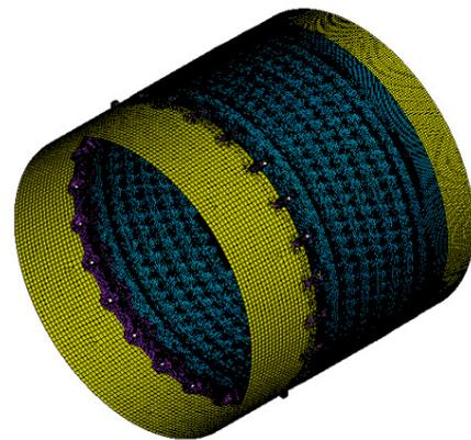
Figure 8: Overall model of the second stage interstage, including adjacent structures
