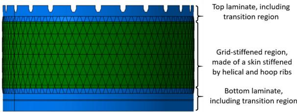
Figure 6: Short interstage design, cut view from inside
