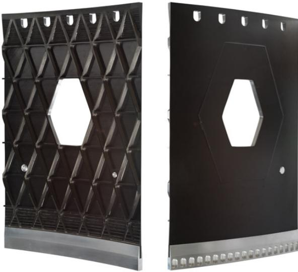
Figure 1: Grid-stiffened conical panel demonstrator
