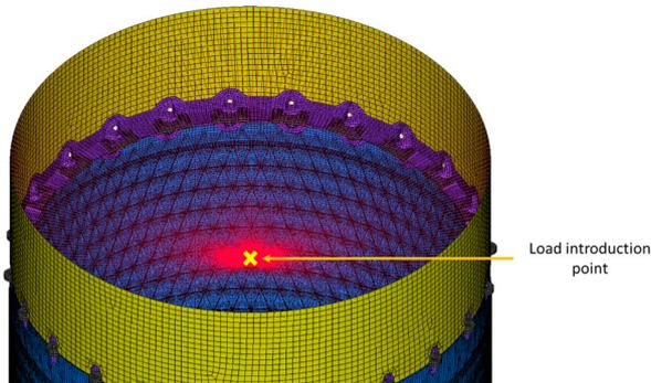
Figure 10: RBE2 element and load introduction point at the top of the composite cylinders
